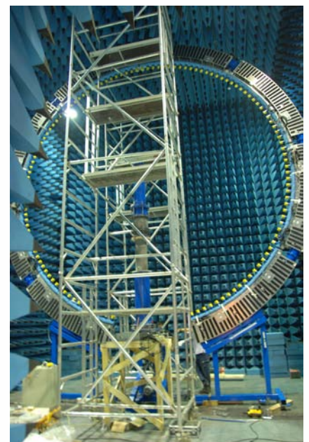
Summitek PIM test equipment and Microwave anechoic chamber
