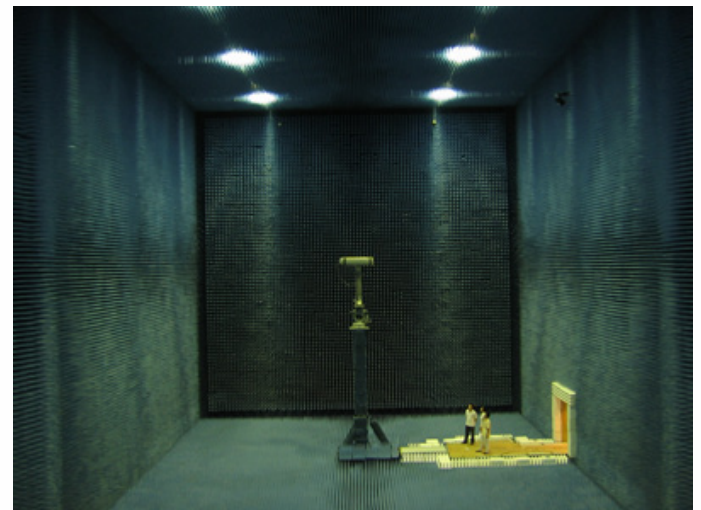
Summitek PIM test equipment and Microwave anechoic chamber
