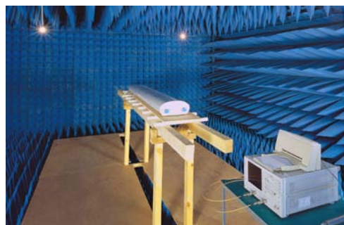
Summitek PIM test equipment and Microwave anechoic chamber
