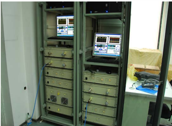
Summitek PIM test equipment and Microwave anechoic chamber
